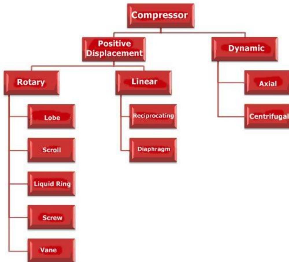
Figure 1. Compressor Types
