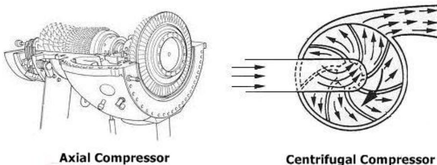
Figure 7. General Structure of Dynamic Compressors
