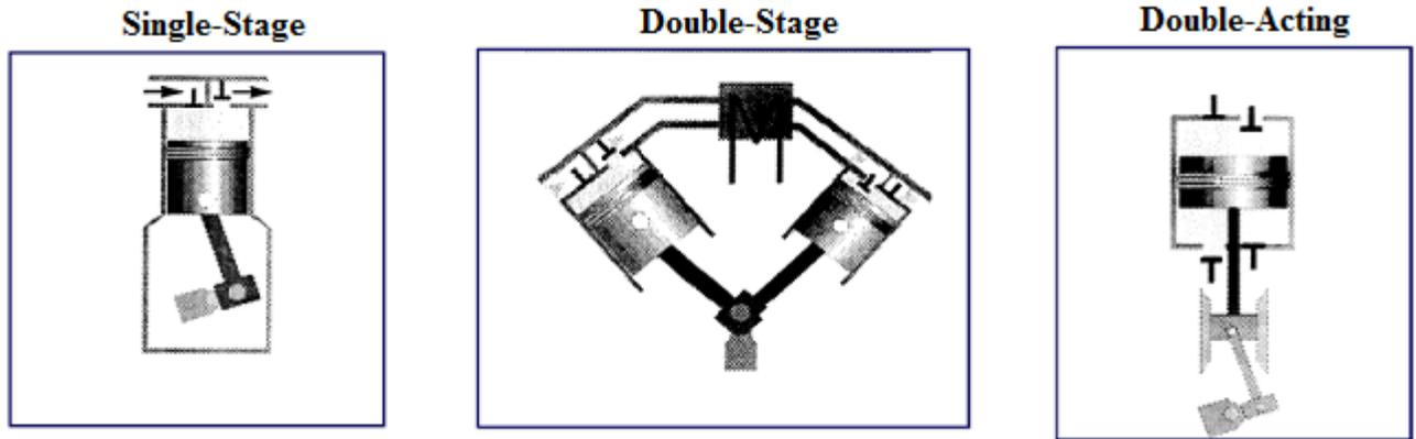
Figure 6. Types of Reciprocating Compressors
