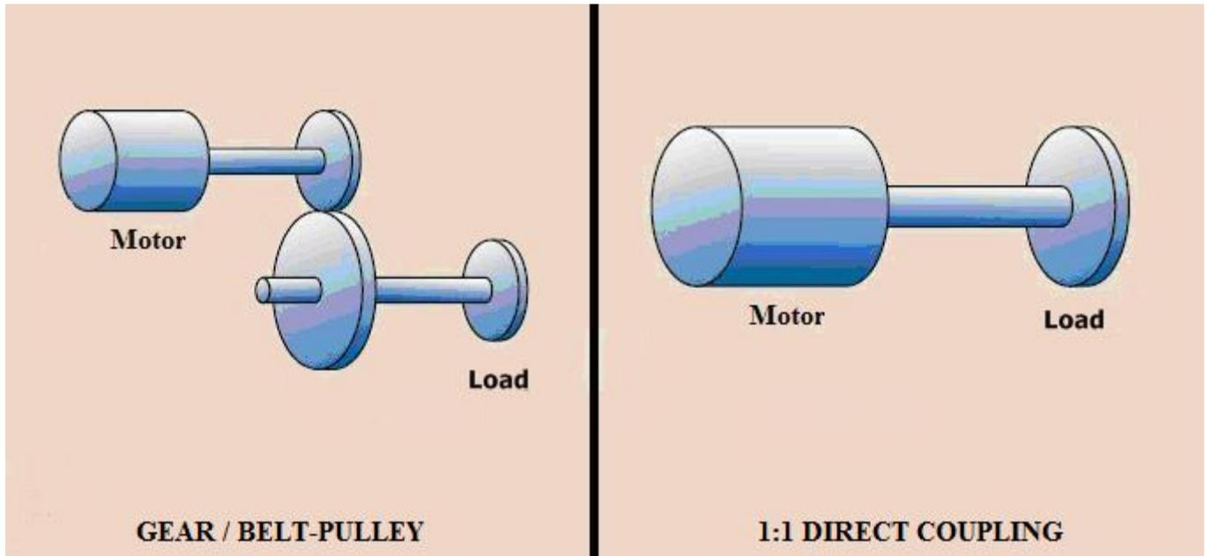
Figure 8. Motor Power Transmission Types
