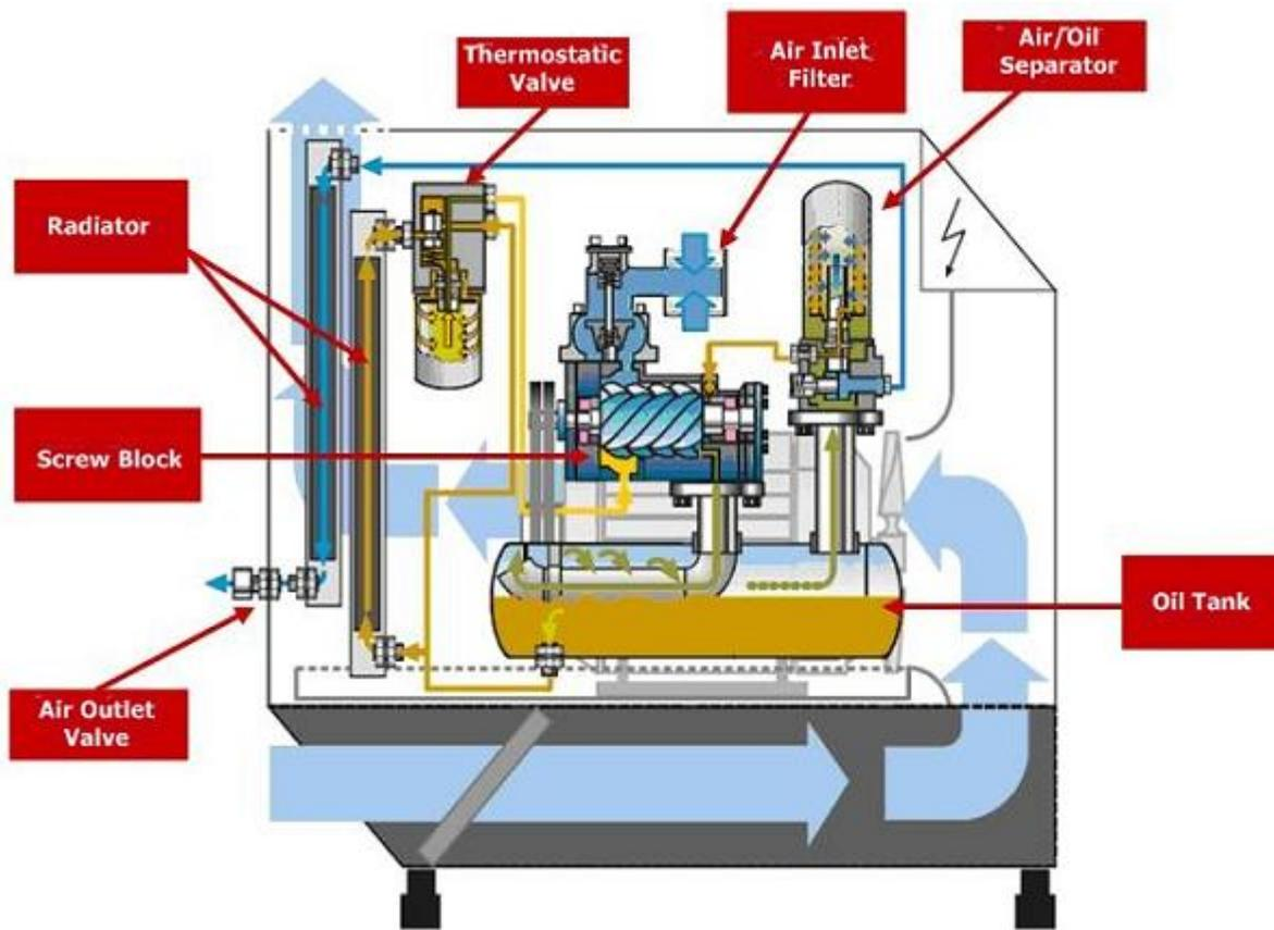
Figure 4. The Structure of an Oil Injected Screw Compressor
