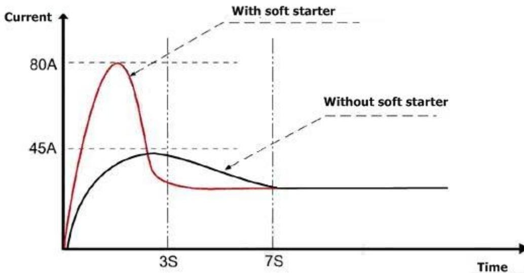
Figure 10. Impact of the Soft Starter on the Motor Startup Current
