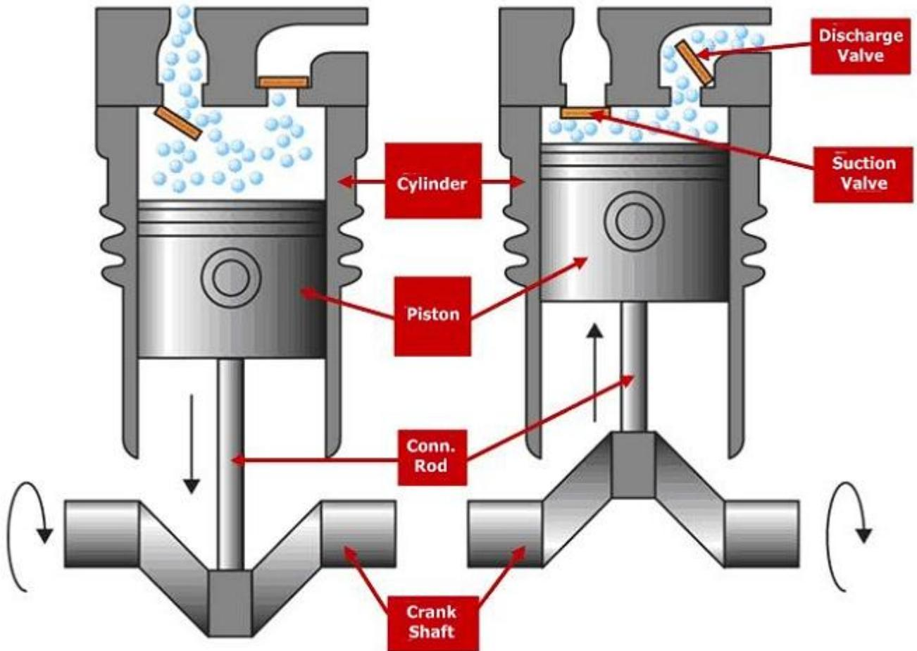
Figure 5. Structure of a Reciprocating Compressor
