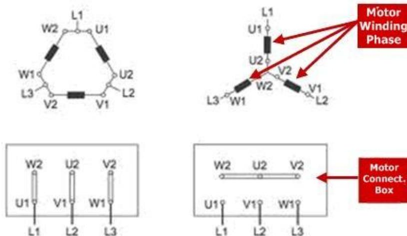
Figure 9. Star-Delta Motor Connection
