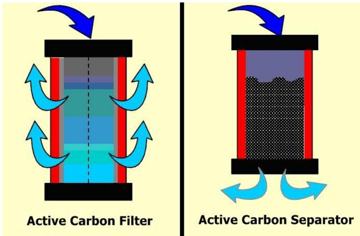
**Figure 21. Oil Filtration Equipment**
