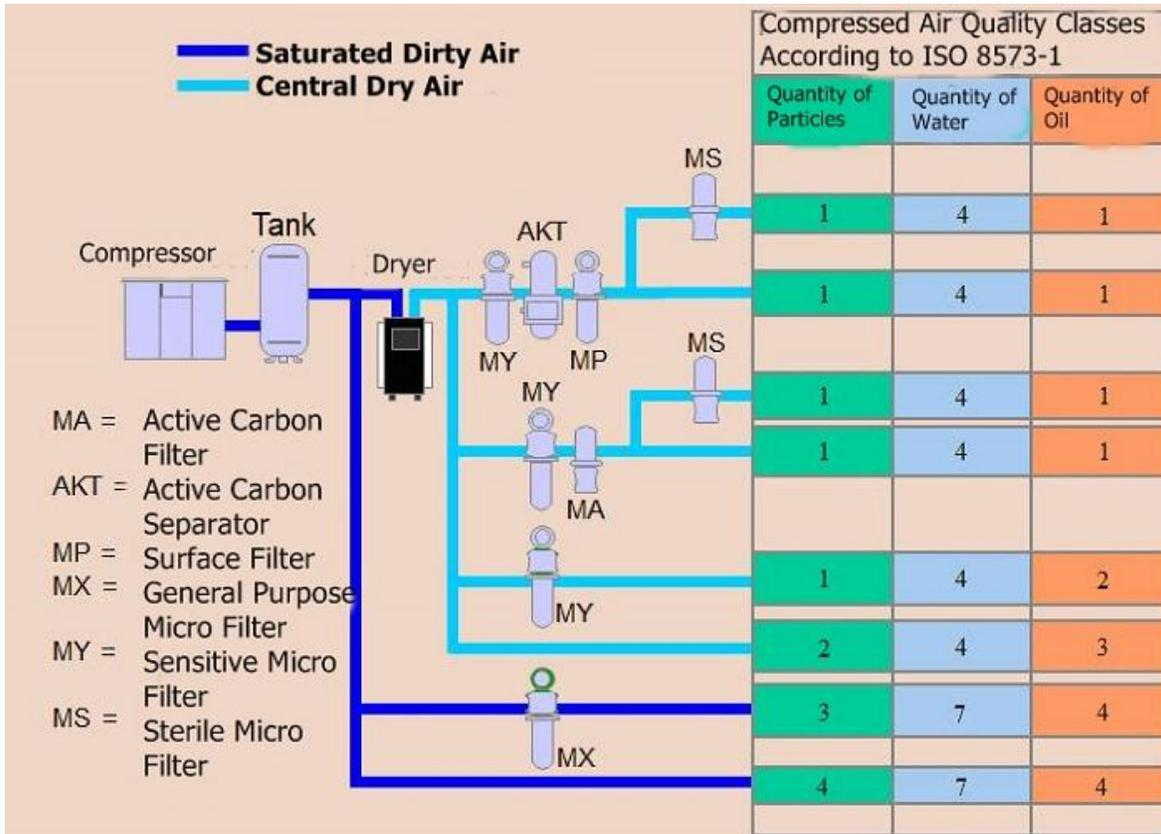
**Figure 22.** Air Quality Classes by Refrigerant Dryers
