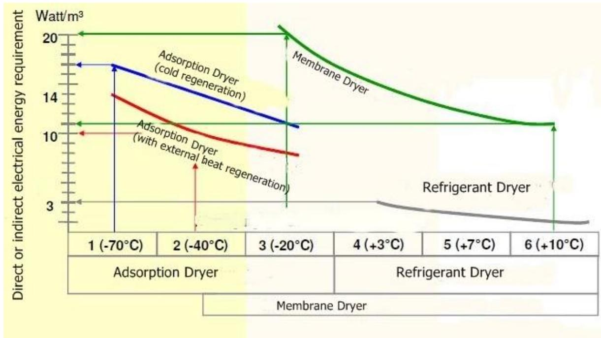
**Figure 14. Pressurized Dew Point Classes of Dryers**
