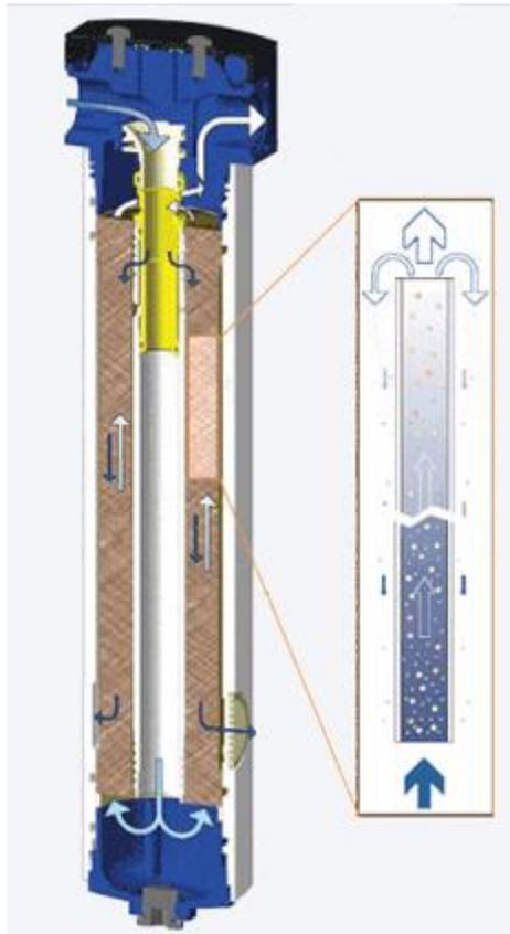
**Figure 17. Structure of Membrane Dryer**
