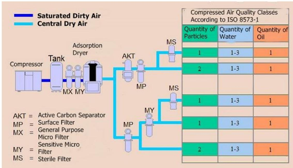
**Figure 23.** Air Quality Classes by Adsorption Dryers
