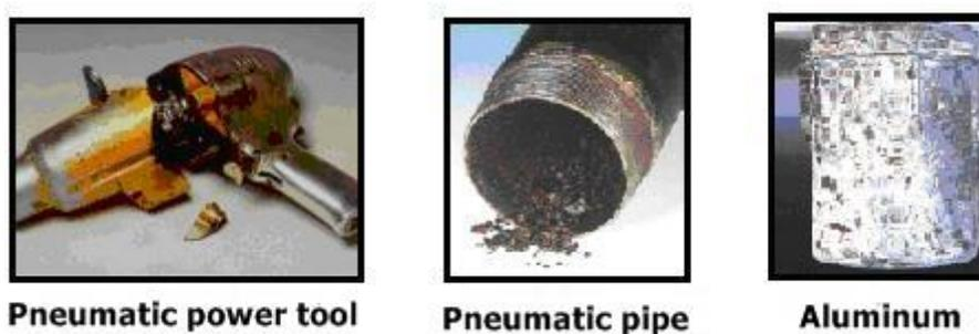
**Figure 13. Consequences of Using Humid Air**
