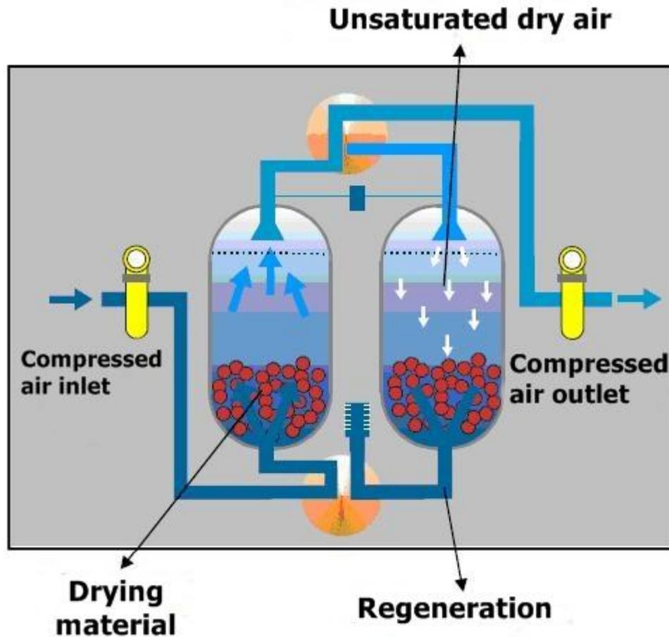
**Figure 16. Structure of Adsorption Dryer**
