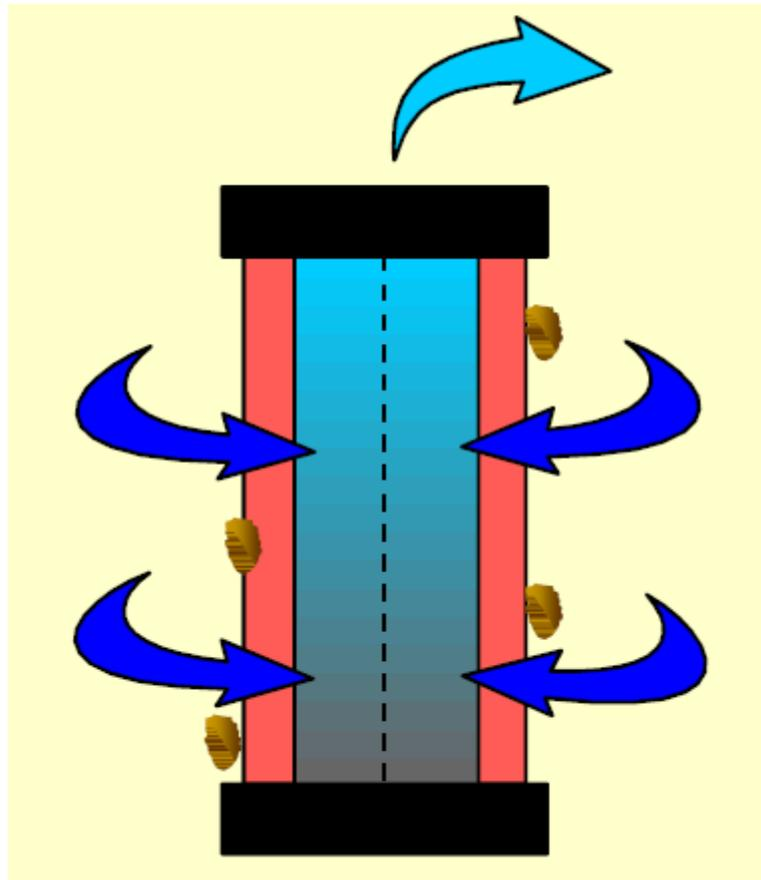
**Figure 19. Structure of a Surface Filter**
