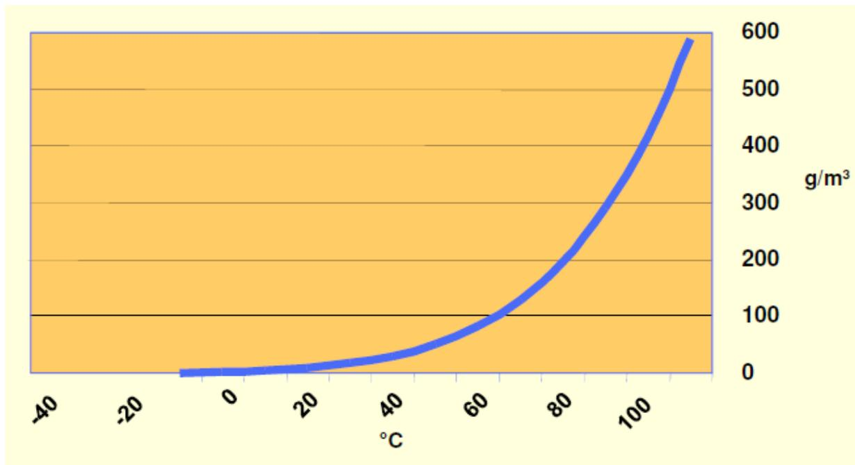
**Figure 12.** Moisture Holding Capacity of Air According to Temperature
