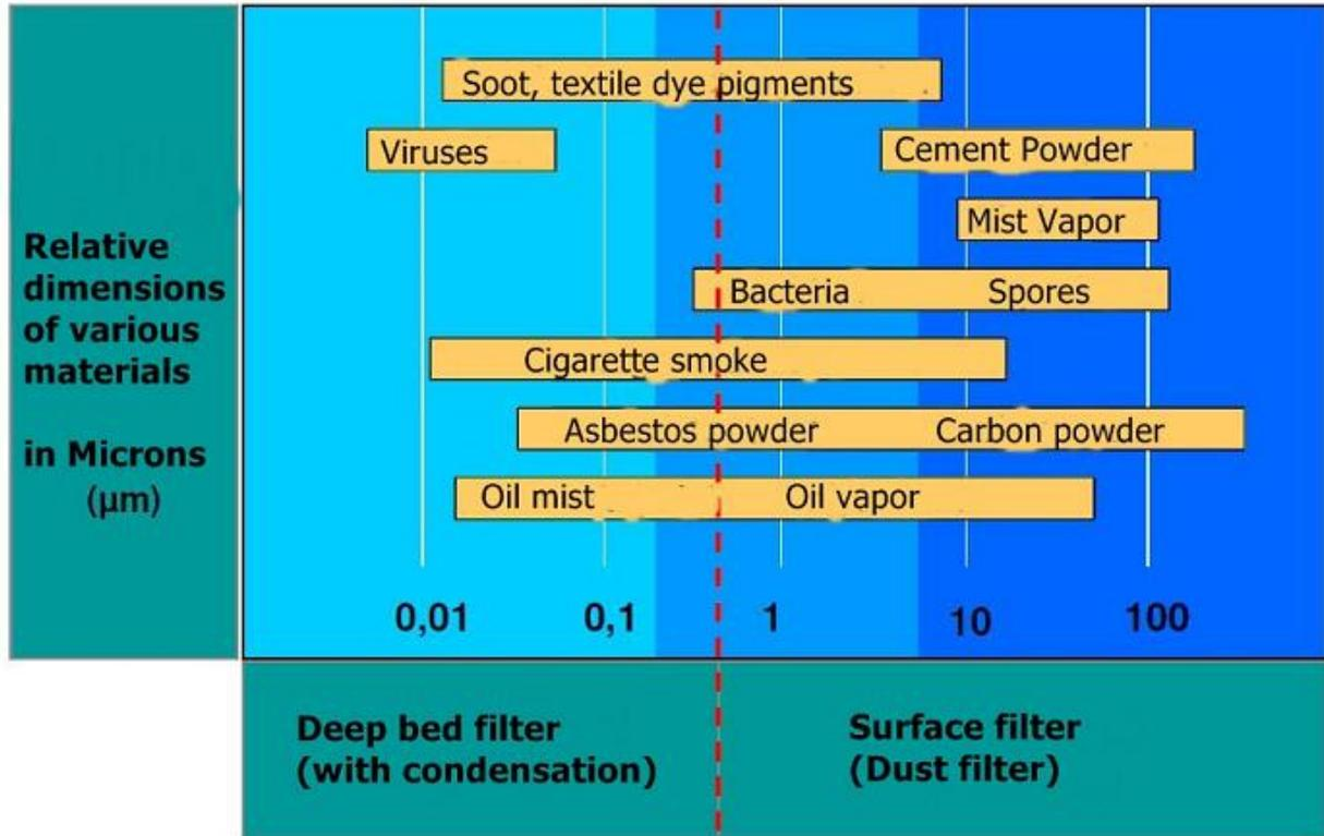
**Figure 18. The Filtration Spectrum**
